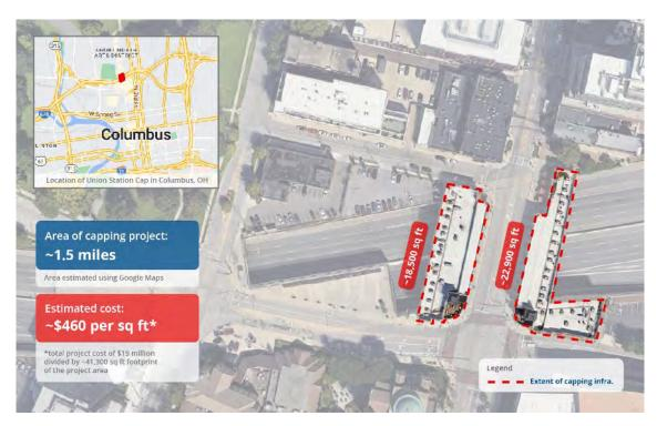
Figure 4.2: Extent of the Union Station Cap in Columbus, OH and total project cost by estimated square footage (Source: FHWA)
