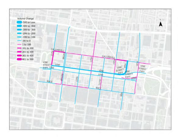
Figure 7: Volume Change - No Build to Build Alternative 2 - PM Peak Hour
