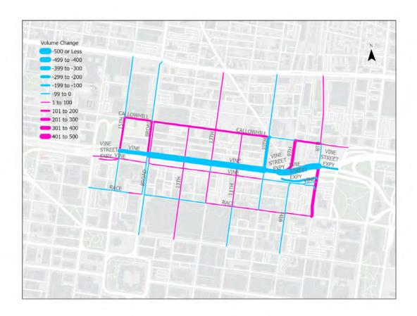
Figure 5: Volume Change - No Build to Build Alternative 1 - PM Peak Hour
